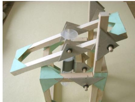
In the Lifter model the effort is applied by a pneumatic cylinder between the fulcrum (the dowel connected to the uprights) and the resistance or load at the end of the arm. If the effort were applied closer to the fulcrum more effort or pneumatic force would be required to lift the same load.
