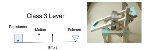
In the Lifter model the effort is applied by a pneumatic cylinder between the fulcrum (the dowel connected to the uprights) and the resistance or load at the end of the arm. If the effort were applied closer to the fulcrum more effort or pneumatic force would be required to lift the same load.
