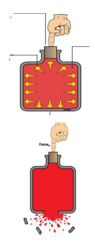
Pascal demonstrated the practical use of his laws with illustrations such as that shown below. This diagram shows how, by applying the same principle described above, a small input force applied against a small area can result in a large force by increasing the output area.
