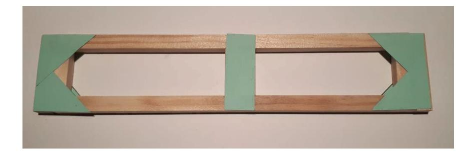
Glue the three  $2\frac{3}{8}$ " – 60mm axles into the holes of a drilled  $3\frac{5}{8}$ " – 90mm piece. The dowels are to be flush with one side and this is covered by a  $3\frac{5}{8}$ " by  $\frac{3}{8}$ " (90mm by 10mm) cardboard strip cut from the green card.
