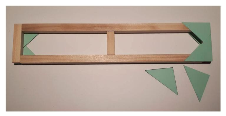
On the other side of the frame glue two  $1\frac{1}{4}$ " – 32mm pieces into the smaller ends. Secure them with glue and with four corner gussets, one on each corner.
