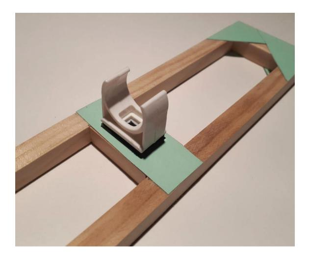
Attach the second 3<sup>5</sup>/<sub>8</sub>" - 90mm piece to the dowels so that the pieces are on different sides of the frame. The assembly should slide freely.
