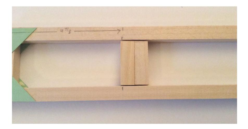
From the green gusset card cut a rectangle  $\frac{3}{4}$ " by 2" – (19mm by 51mm) and glue it to secure the two  $1\frac{1}{4}$ " – 32mm pieces to the frame.
