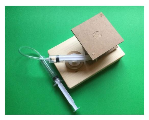
The rotation of the platform will be approx. 40°. The pressure inside the syringes, operated pneumatically, is insufficient to overcome the force the clip places on the barrel of the syringe in the structure.
